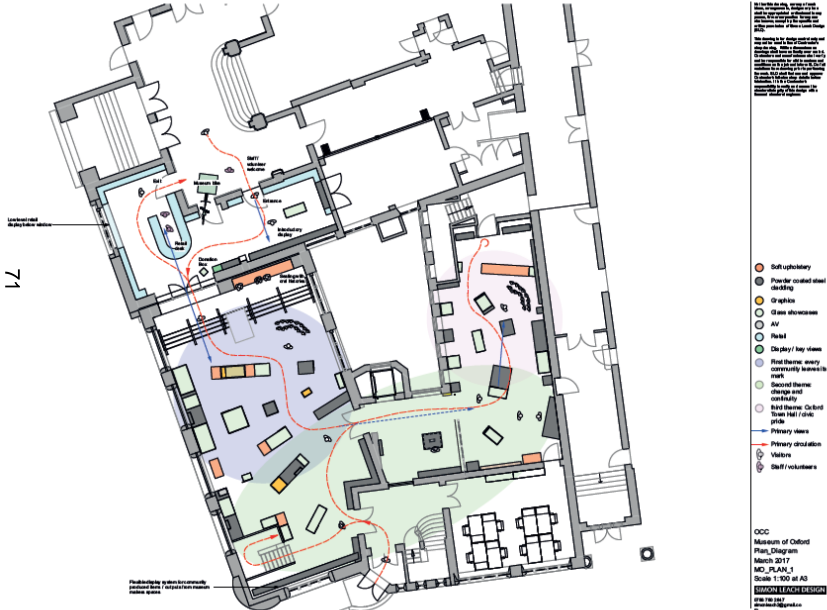
Drawing 3- Exhibition fit out design, ground floor
